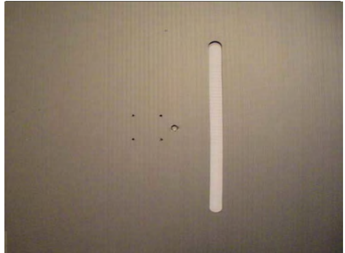
Motor mount and wire holes.
