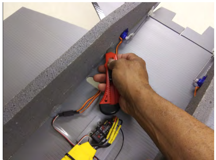
Cut slot in left nacelle for servo wire and extension, single knife cut is sufficient here.
